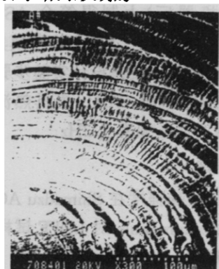
Fig. 3 Multi-layer structure of the fracture surface of self-reinforced LDPE
